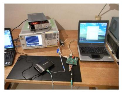
Transmitter Radiated Spurious Emissions (RF Radiated test)
