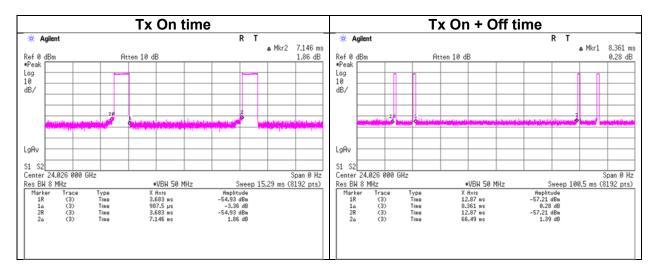
There are two doppler frequencies and chirp part in one transmission period. These doppler parts and chirp part were compared to calculate the duty factor. The duty factor was calculated within doppler part, because doppler's dwell time is longer than the chirp part.
