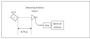
Distance Factor:  $20 \times \log (0.75 \text{ m}^* / 3.0 \text{ m}) = -12.0 \text{ dB}$ \*Test Distance: 0.75 m
