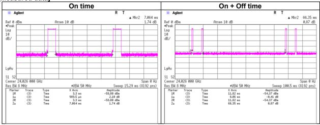
There are two doppler frequencies and chirp part in one transmission period. These doppler parts and chirp part were compared to calculate the duty factor. The duty factor was calculated within doppler part, because doppler's dwell time is longer than the chirp part.
