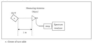
Distance Factor:  $20 \times (1.0 \text{ m}^* / 3.0 \text{ m}) = -9.5 \text{ dB}$
