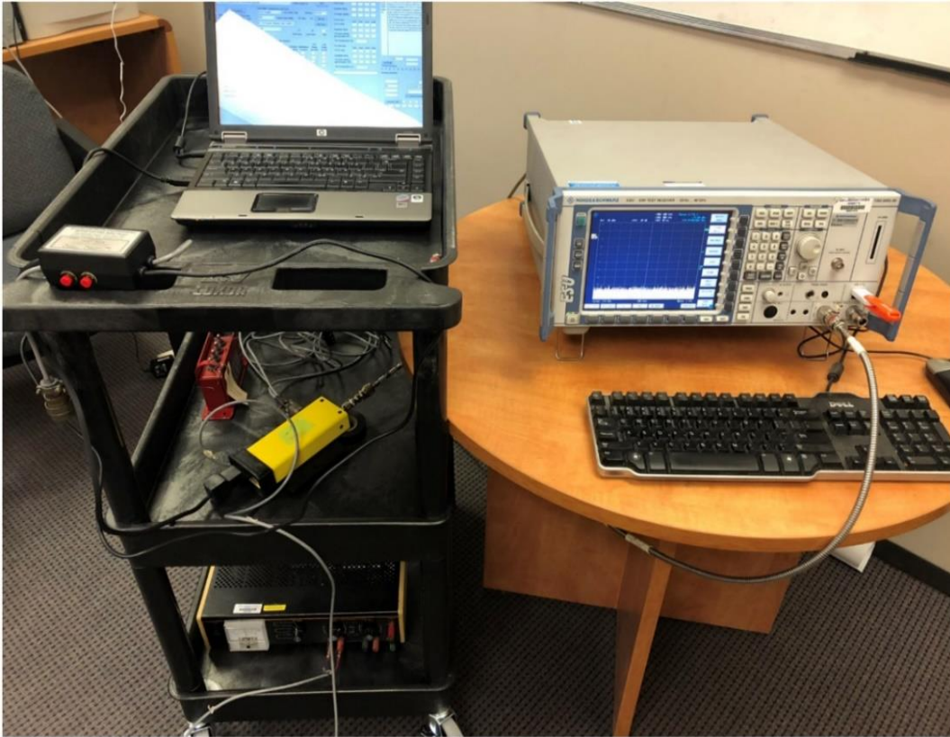
Conducted Radio Measurement Setup – Photo1
