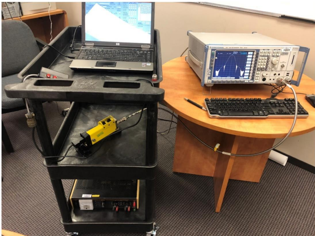
Conducted Radio Measurement Setup – Photo2
