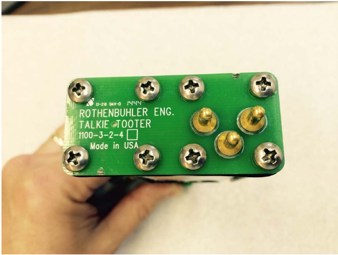
Picture 9 1100-3-2 Internal Assembly Charger Interface End View
