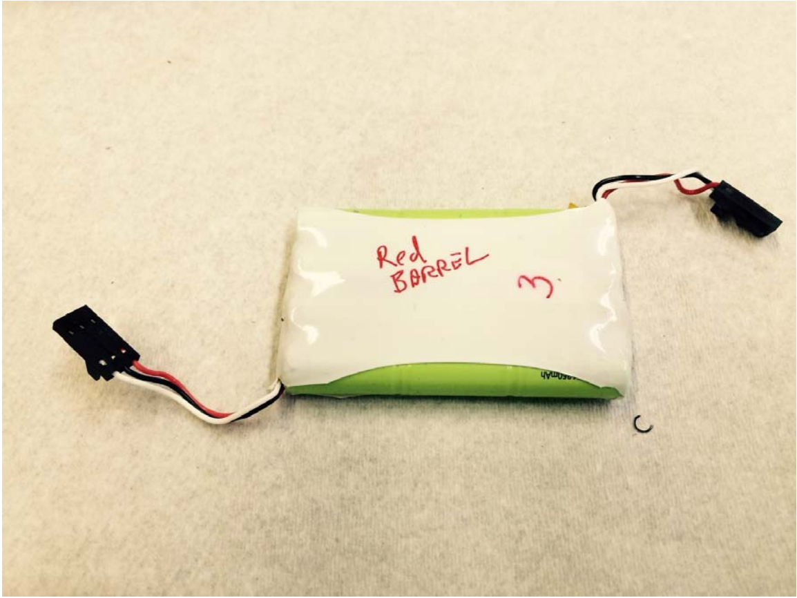
Picture 16 1100-2-6 Battery Pack, 14.4V 350mAH NiMH
