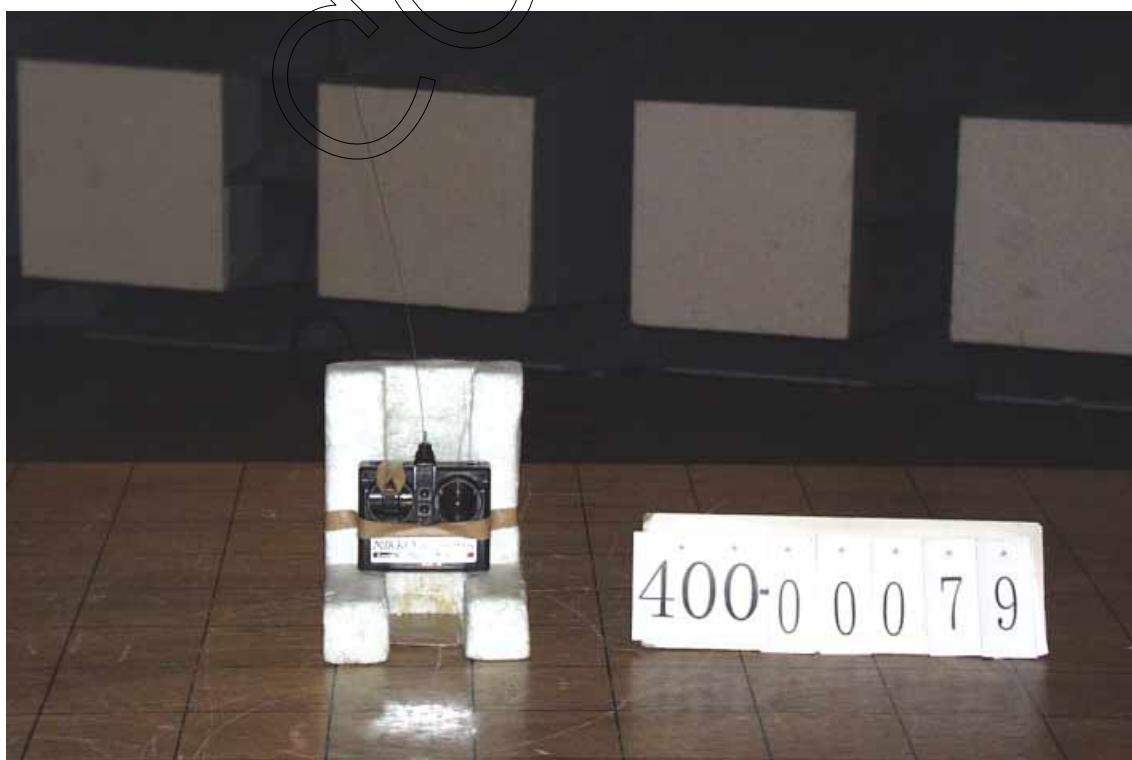
**TEST DATA****2.2 Radiated Emissions Measurement**Date : May 17, 2000Temp.: 24 °C Humi.: 62 %
