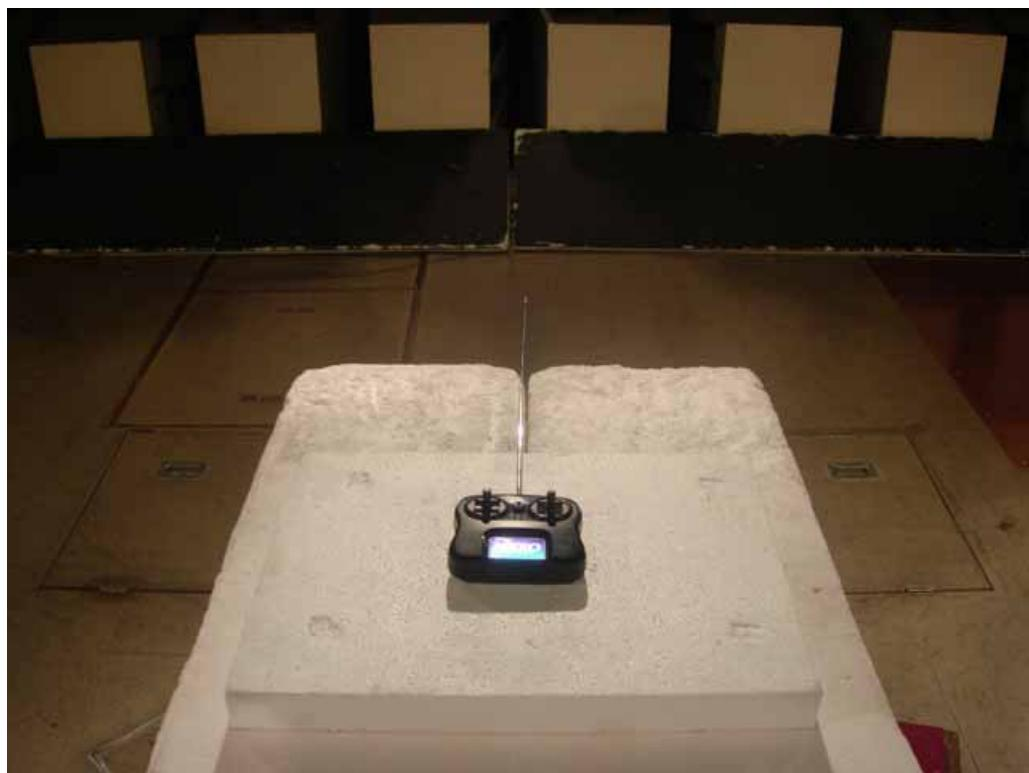
**PHOTOGRAPHS OF EUT CONFIGURATION FOR RADIATED EMISSIONS MEASUREMENT**
