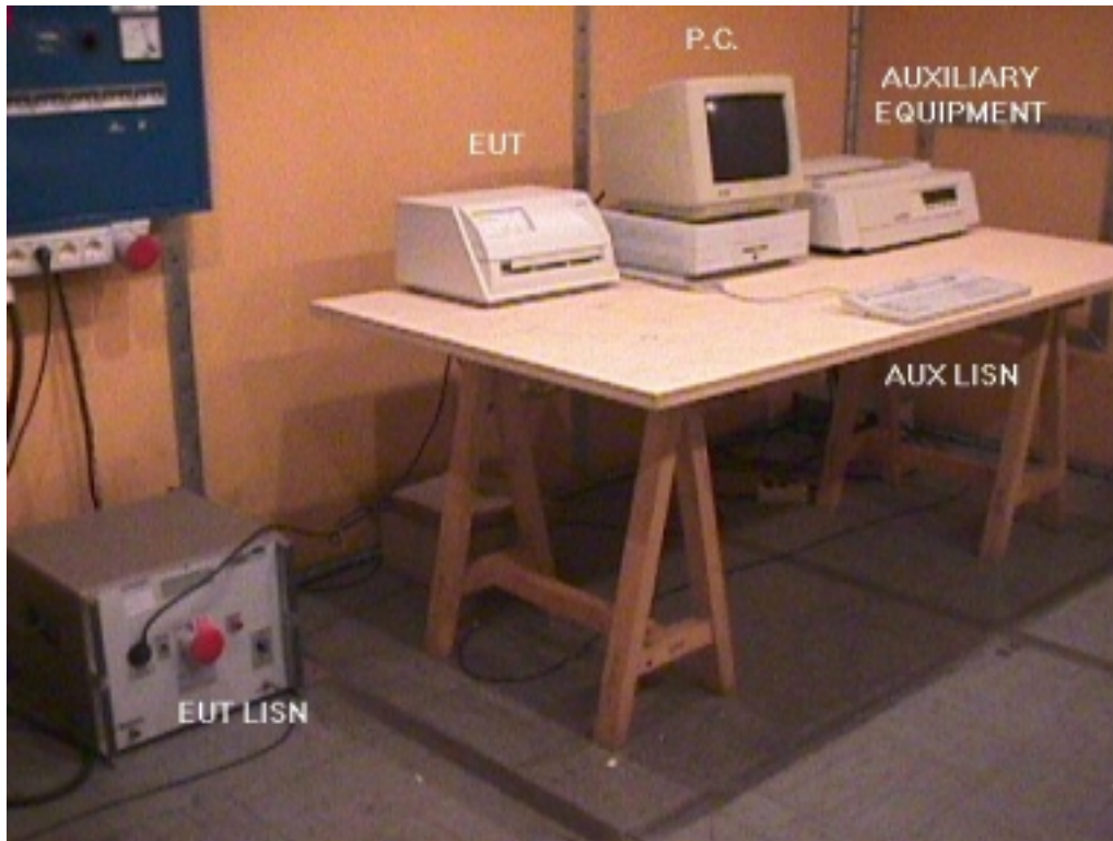
picture 1: conducted measurement front view
