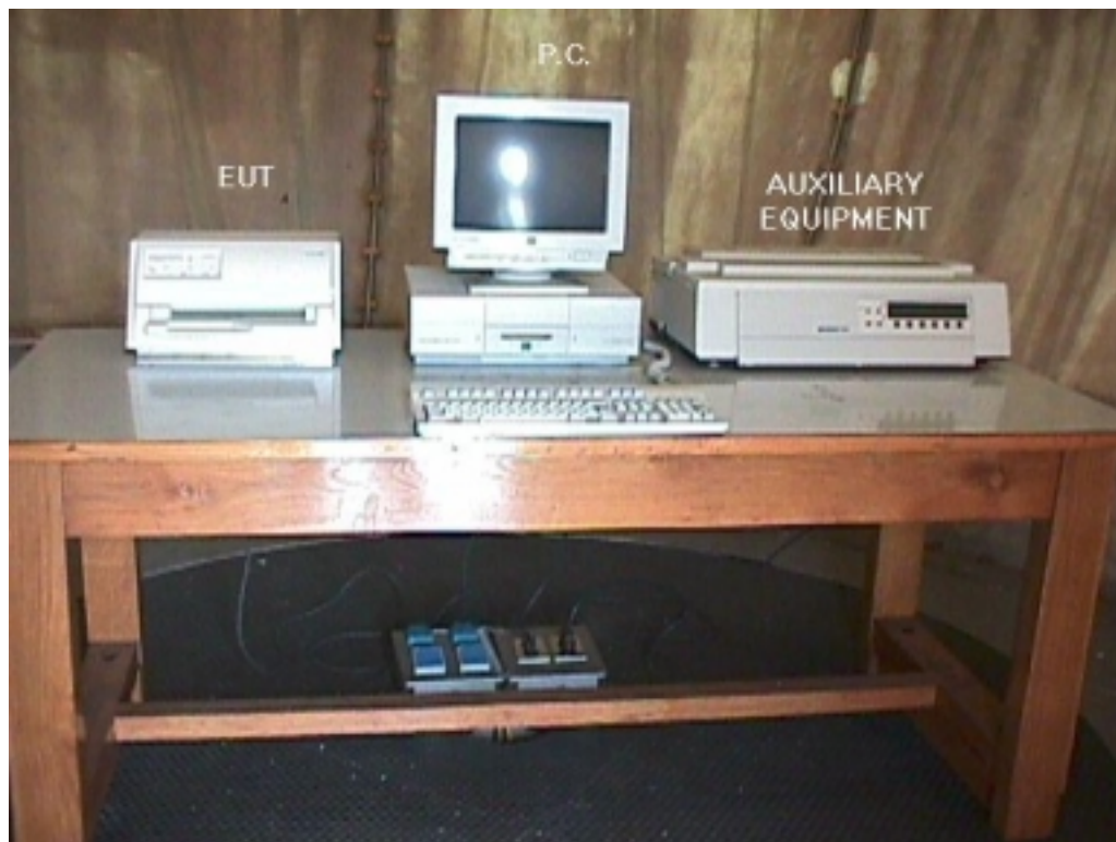
picture 4: radiated measurements front view
