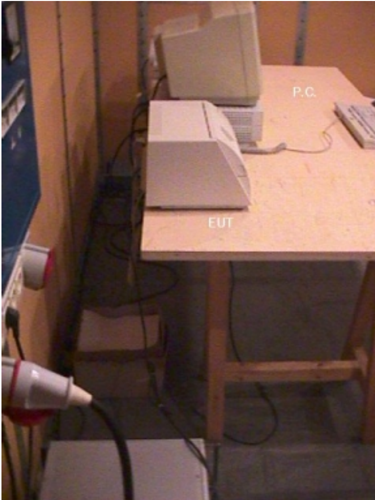
picture 3: conducted measurement rear view parallel transmission
