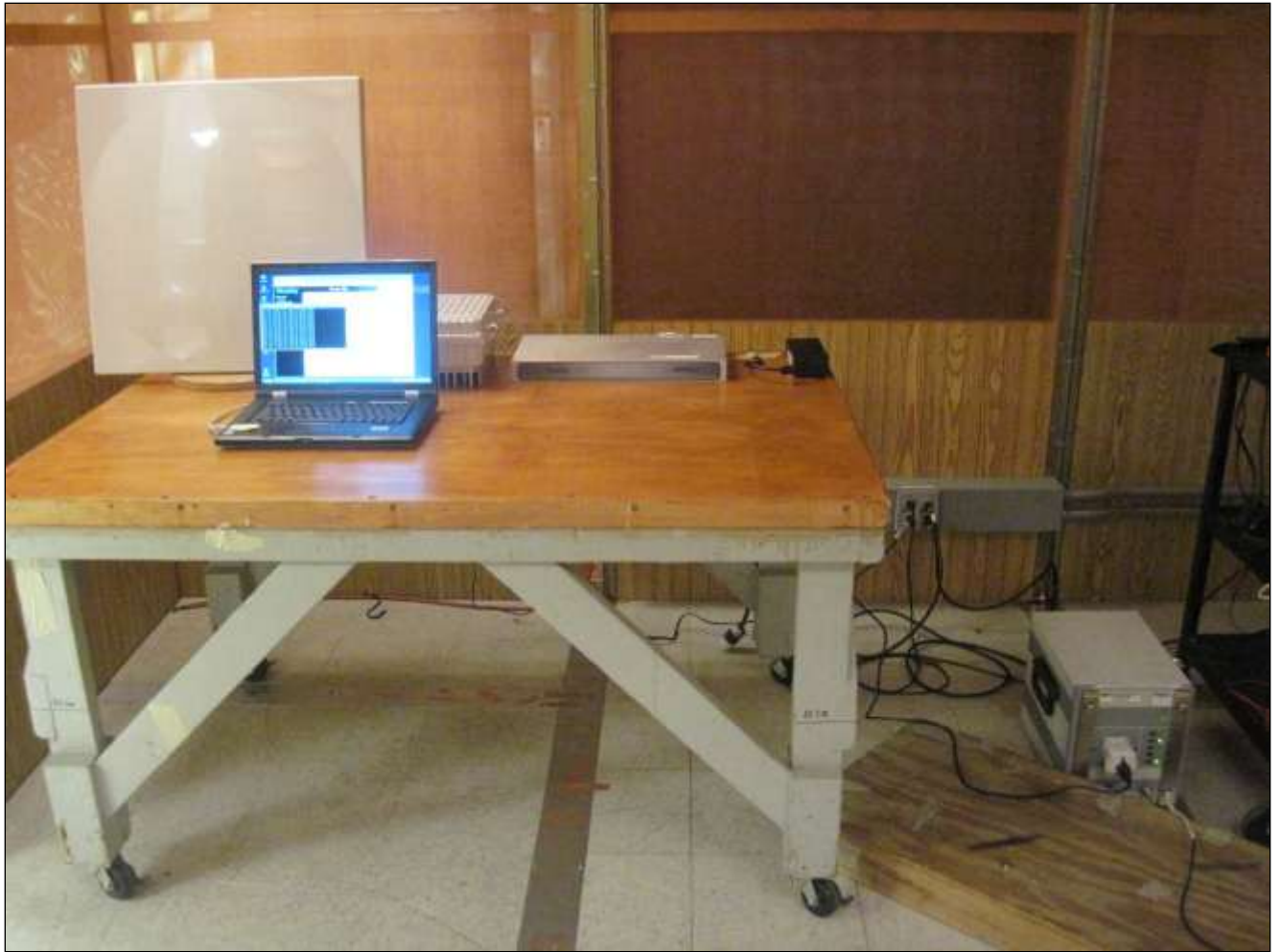
Photograph 1. Conducted Emissions, Test Setup
