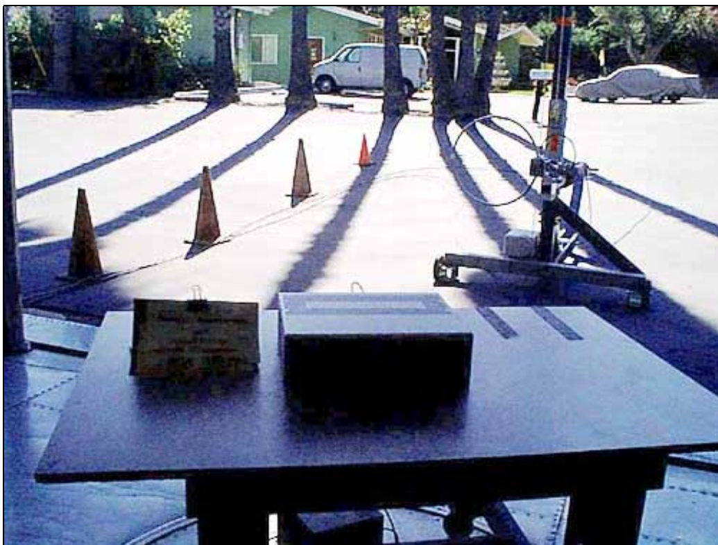
Radiated Emissions - Front View - With Loop Antenna
