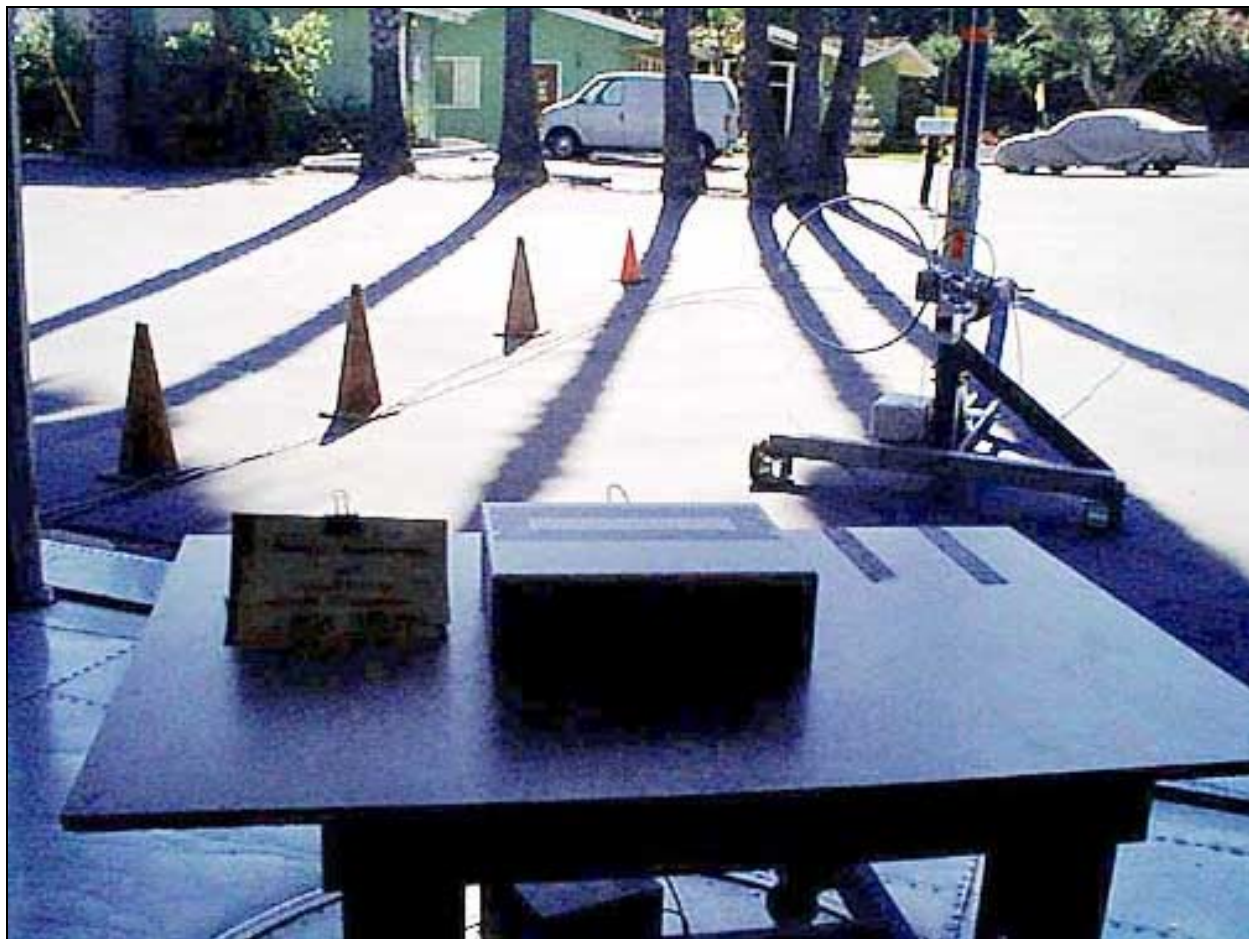
Radiated Emissions - Front View - With Loop Antenna
