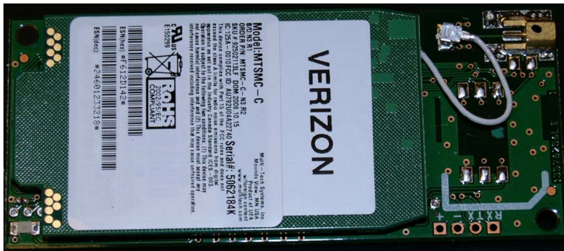
Photo 20: HomeBase (HB-100) – Verizon CDMA Modem PCB – top side
