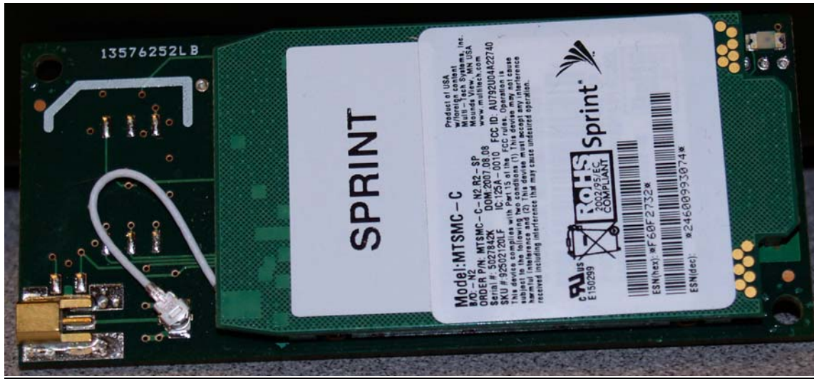
Photo 18: HomeBase (HB-100) – Sprint CDMA Modem PCB – top side
