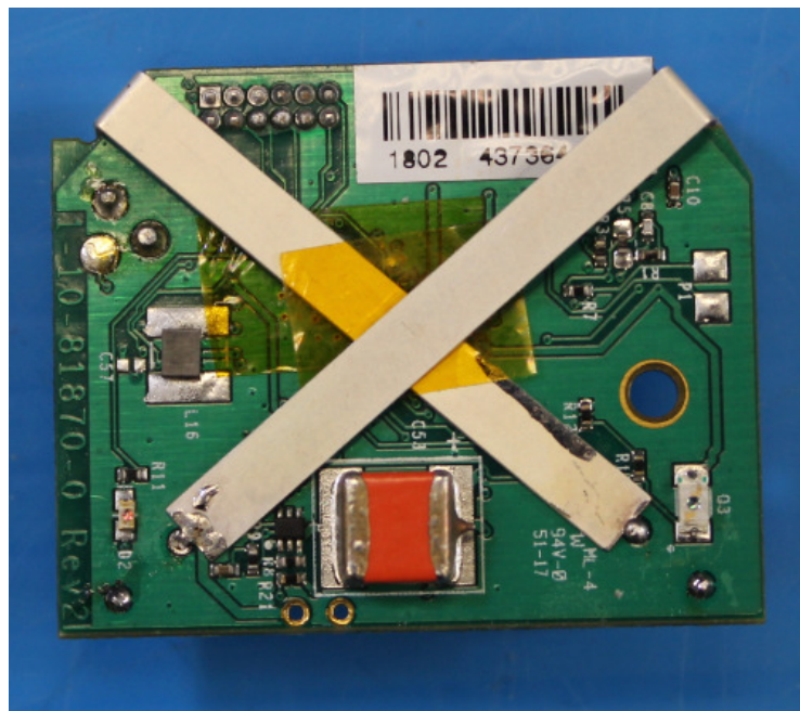
Pic 4 – BI HomeGuard 20/20 Transmitter board bottom Side with antenna installed
