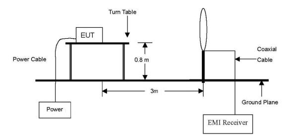
The diagram below shows the test setup that is utilized to make the measurements for emission from 30 Mz to 1  $\mathbb{G}$  Emissions.
