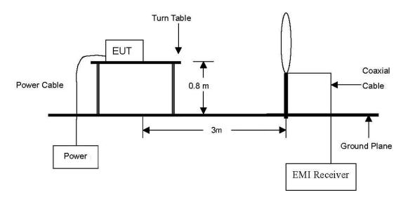
The diagram below shows the test setup that is utilized to make the measurements for emission from 30  $\,\mathrm{Mz}$  to 1  $\,\mathrm{GHz}$ .
