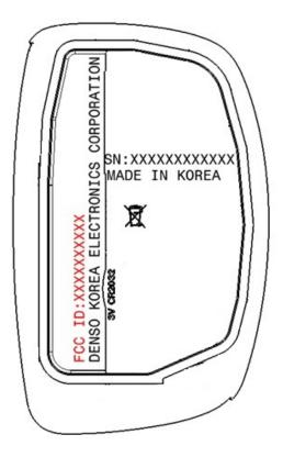
X Product label with FCC ID is affixed on the battery compartment and battery will not be installed when placing to the market. FCC ID will be visible at the time of installing the battery by the user.
