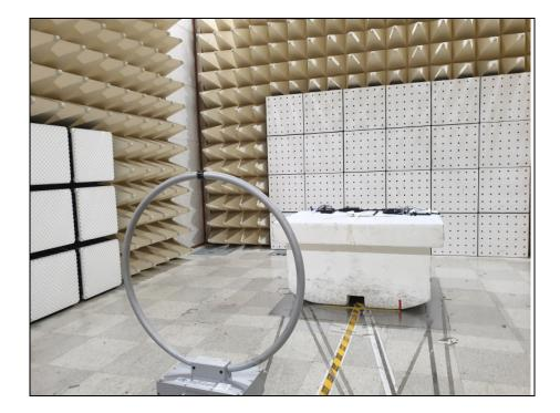
B. Photo of Radiated Spurious Emission Test (Above 30 MHz)
