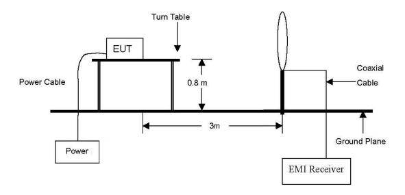
The diagram below shows the test setup that is utilized to make the measurements for emission from 30  $\,\text{Mb}$  to 1  $\,\text{GHz}$ .
