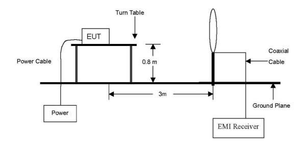
The diagram below shows the test setup that is utilized to make the measurements for emission from 30 Mz to 1 Gz.
