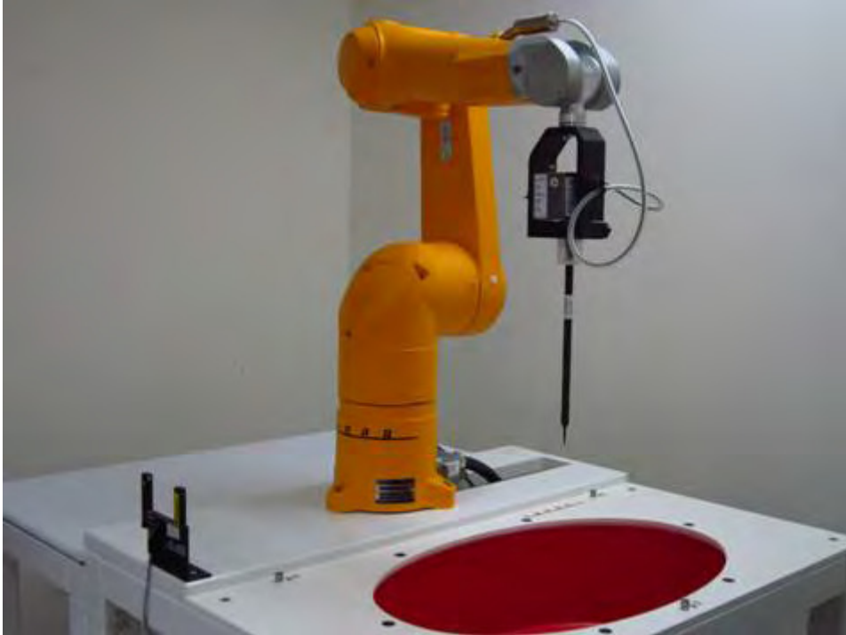
Fig.1 Photograph of the SAR measurement system
