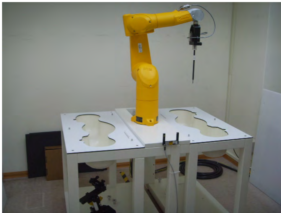
Fig.1 Photograph of the SAR measurement system
