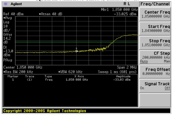
Band edge emission at antenna terminals –15MHz BW LTE-Band 25 (QPSK RB Number: 75 Offset: 0) Channel Highest
