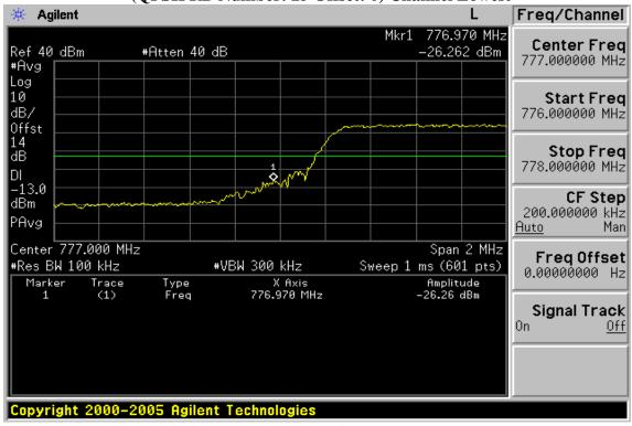
Band edge emission at antenna terminals –5MHz BW LTE-Band 13 (QPSK RB Number: 25 Offset: 0) Channel Highest
