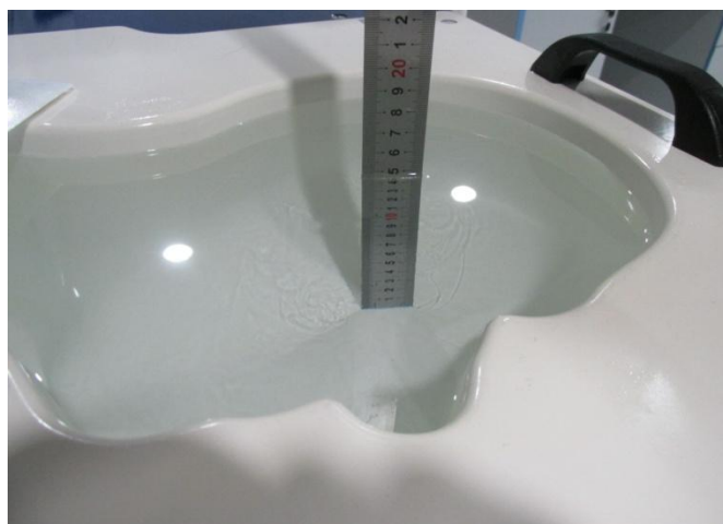
Fig.18 Head Liquid of 2450MHz(15cm)
