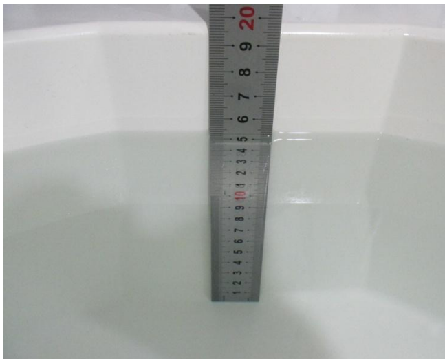
Fig.19 Body Liquid of 2450MHz(15cm)
