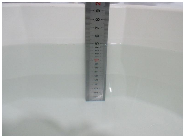
Fig.16 Head Liquid of 1900MHz(15cm)
