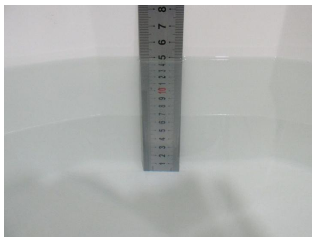
Fig.15 Body Liquid of 1800MHz(15cm)
