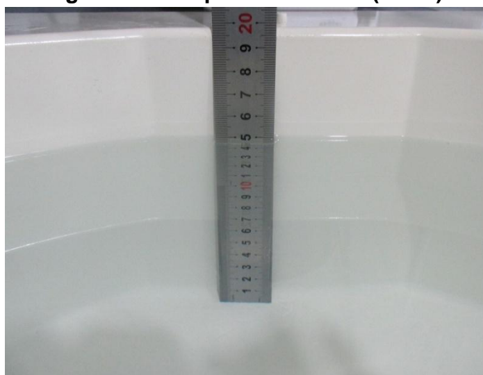
Fig.17 Body Liquid of 1900MHz(15cm)
