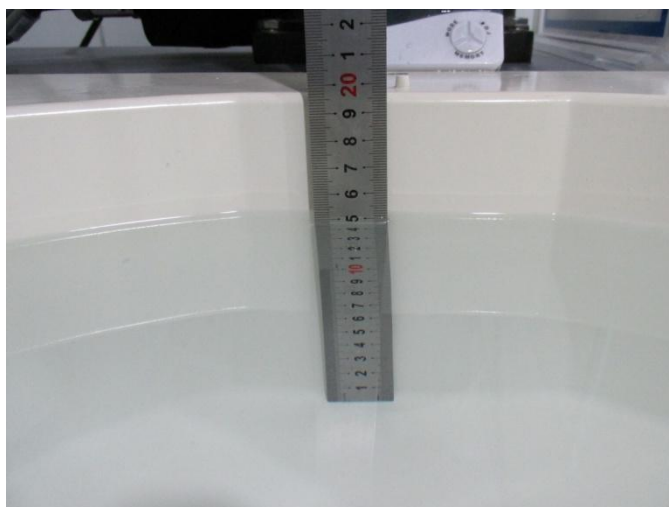
Fig.12 Head Liquid of 835MHz(15cm)
