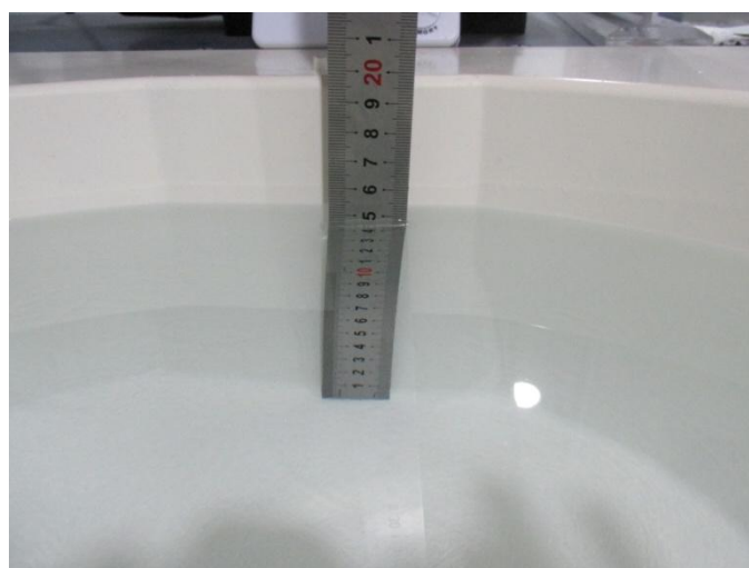
Fig.14 Body Liquid of 835MHz(15cm)
