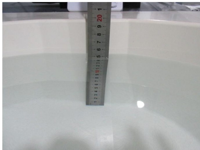
Fig.13 Body Liquid of 835MHz(15cm)
