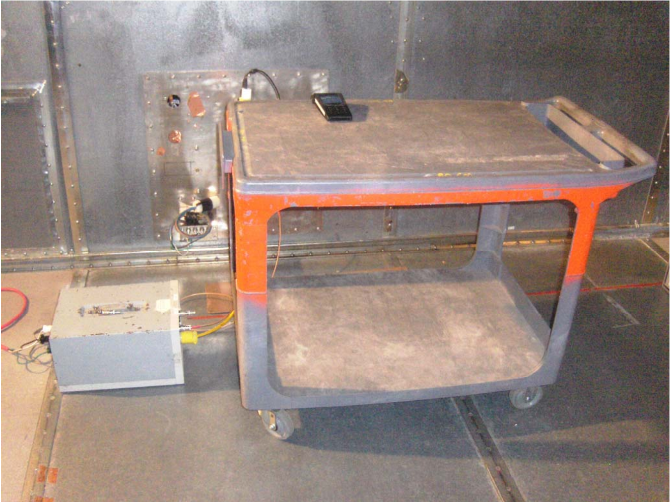
Power Line Conducted Emissions (AC/DC Adaptor)
