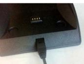
• To charge the terminal, gently place the terminal on to the charging base.
