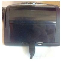
To decrease the charging time, the terminal may be powered off by pressing the key until the display shuts off.
