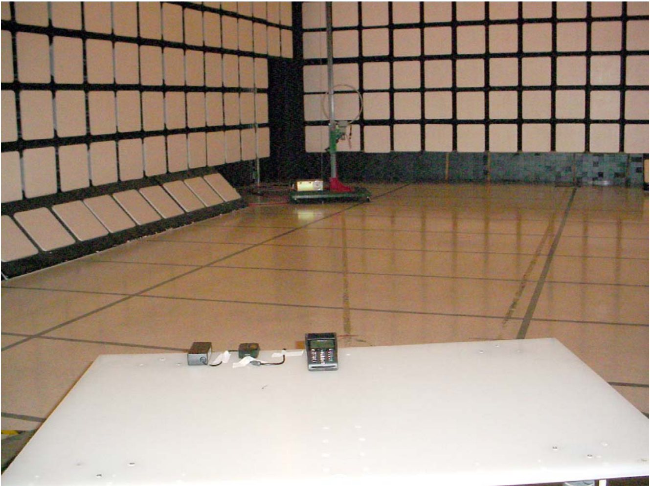
Radiated Emissions @ 10 m – Orthogonal Position 1
