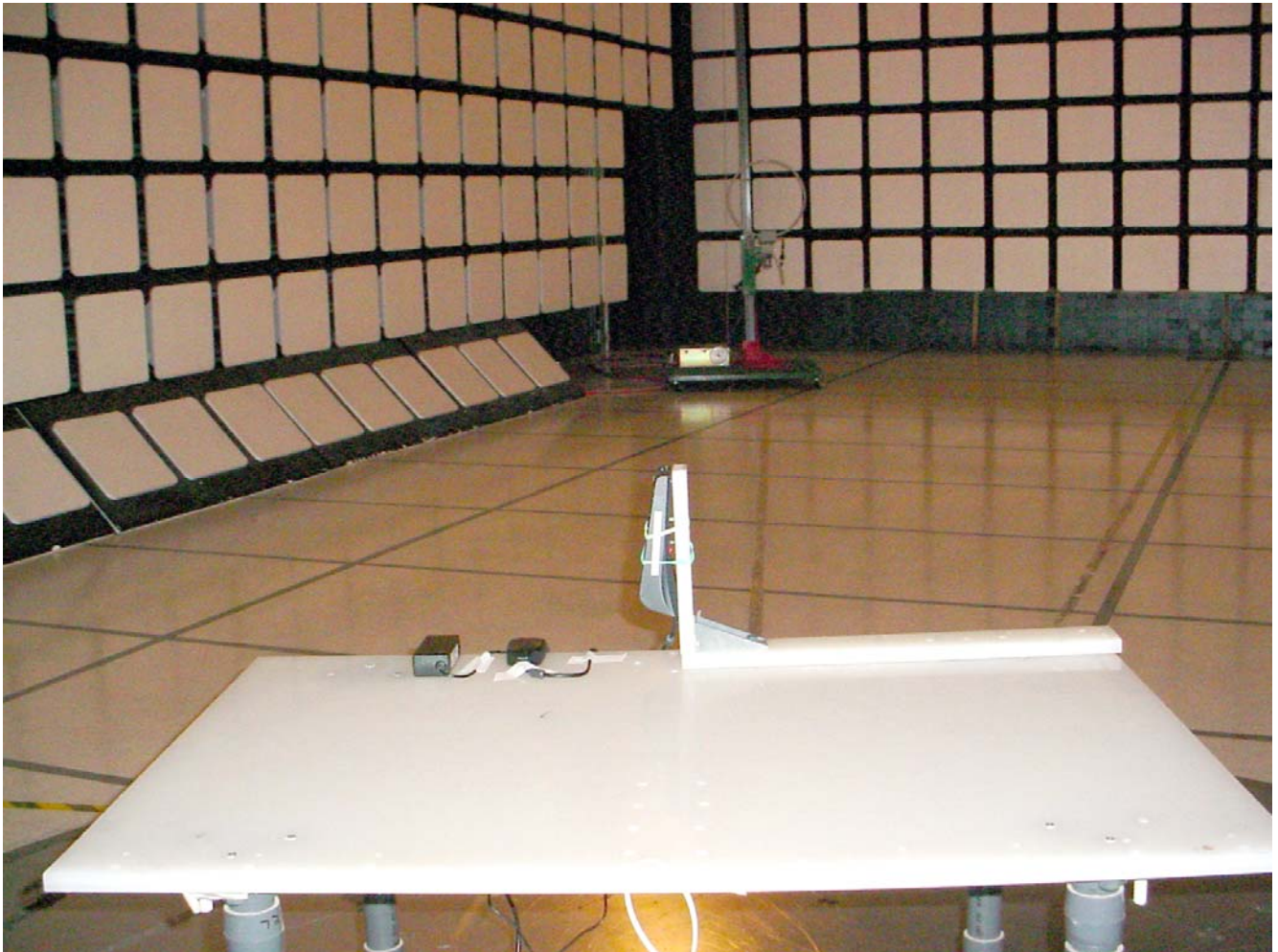
Radiated Emissions @ 10 m – Orthogonal Position 3
