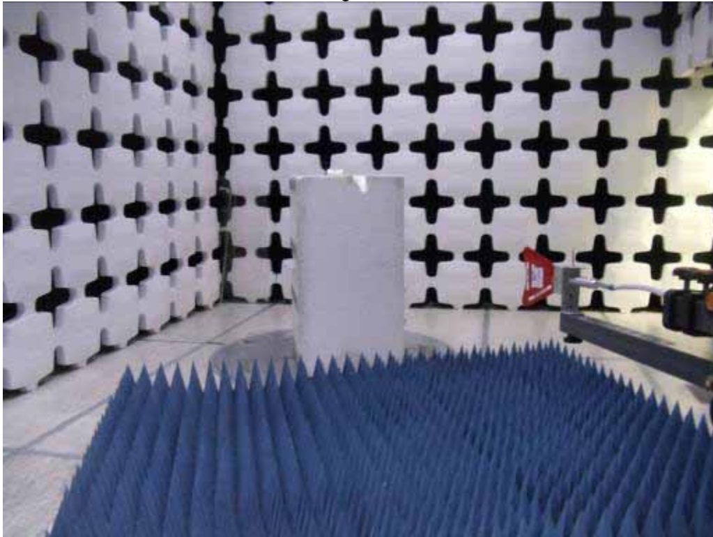
Test Setup for Radiated Spurious Emissions – 1GHz to 10GHz, Horizontal Polarization
