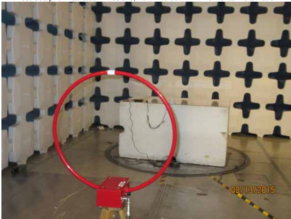
Test Setup for Radiated Emissions, 10kHz to 30MHz – Vertical Polarization
