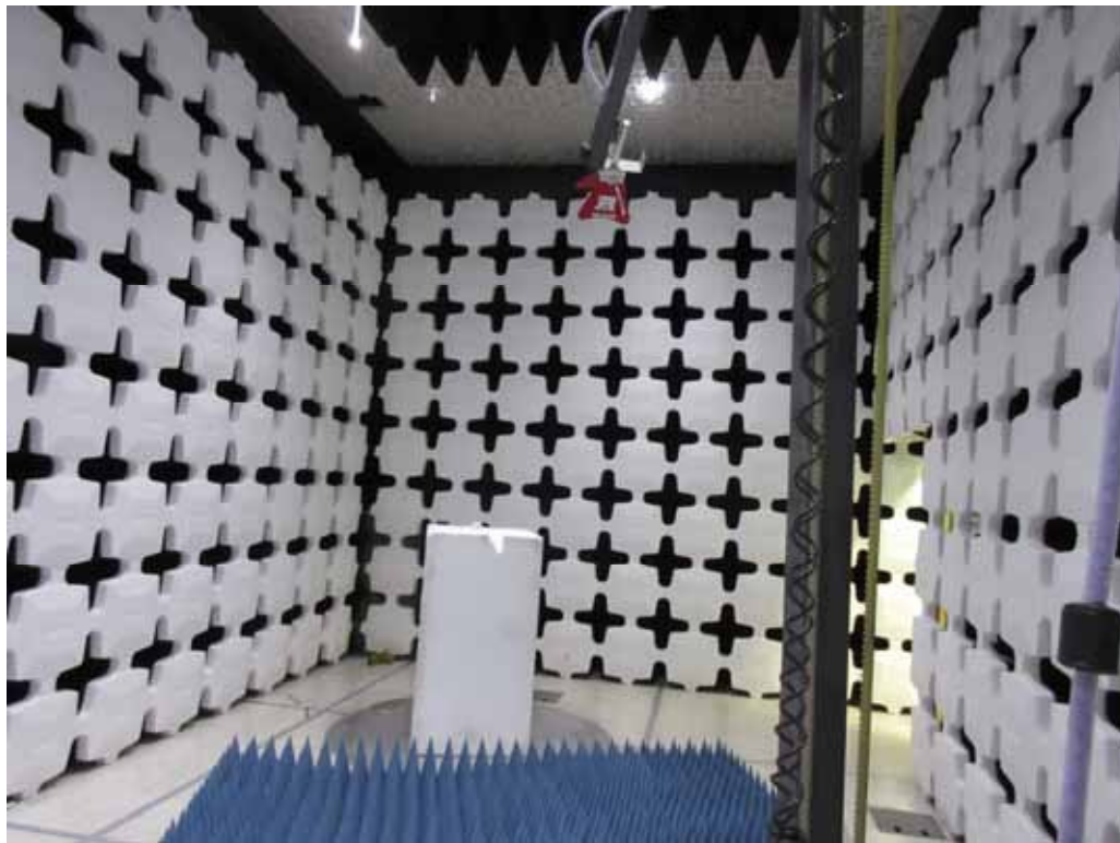
Test Setup for Transmitter Radiated Emissions – 1GHz to 10GHz, Vertical Polarization
