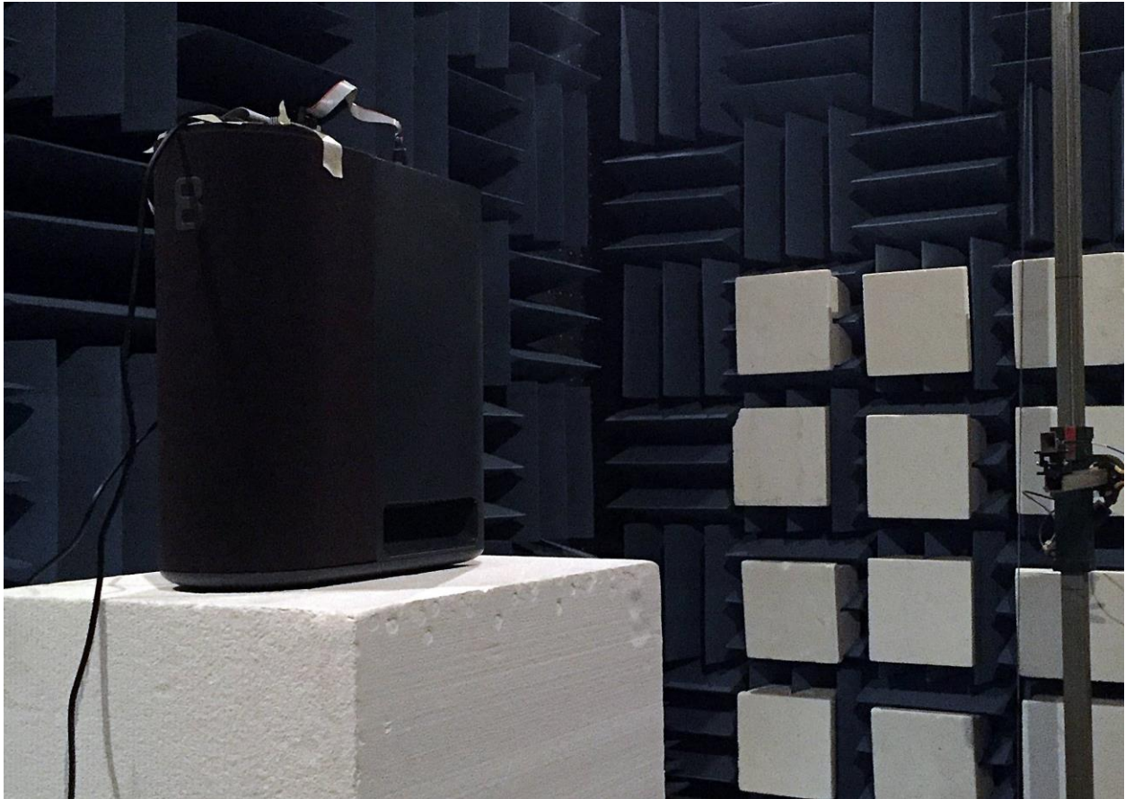
Figure 3: Unwanted Radiated Emissions (18 to 25GHz) Test Setup
