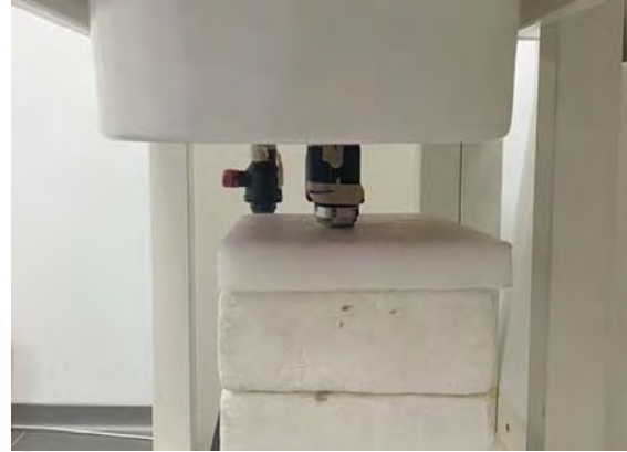
Fig.6 EUT Bottom side to flat phantom
