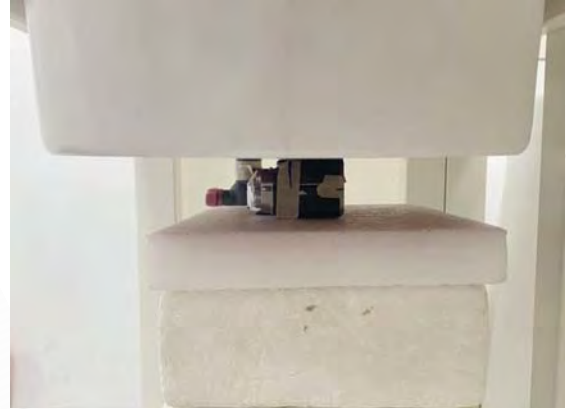
Fig.3 EUT Front side to flat phantom
