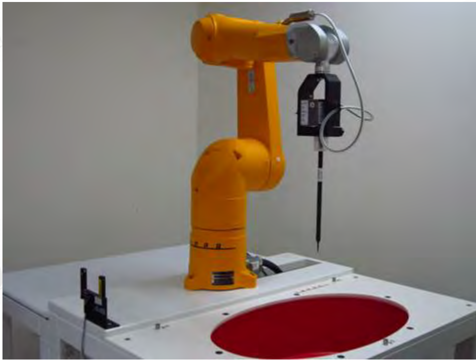
Fig.1 Photograph of the SAR measurement system
