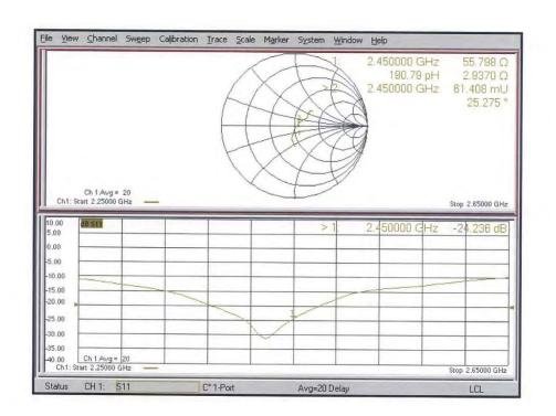
Impedance Measurement Plot for Head TSL
