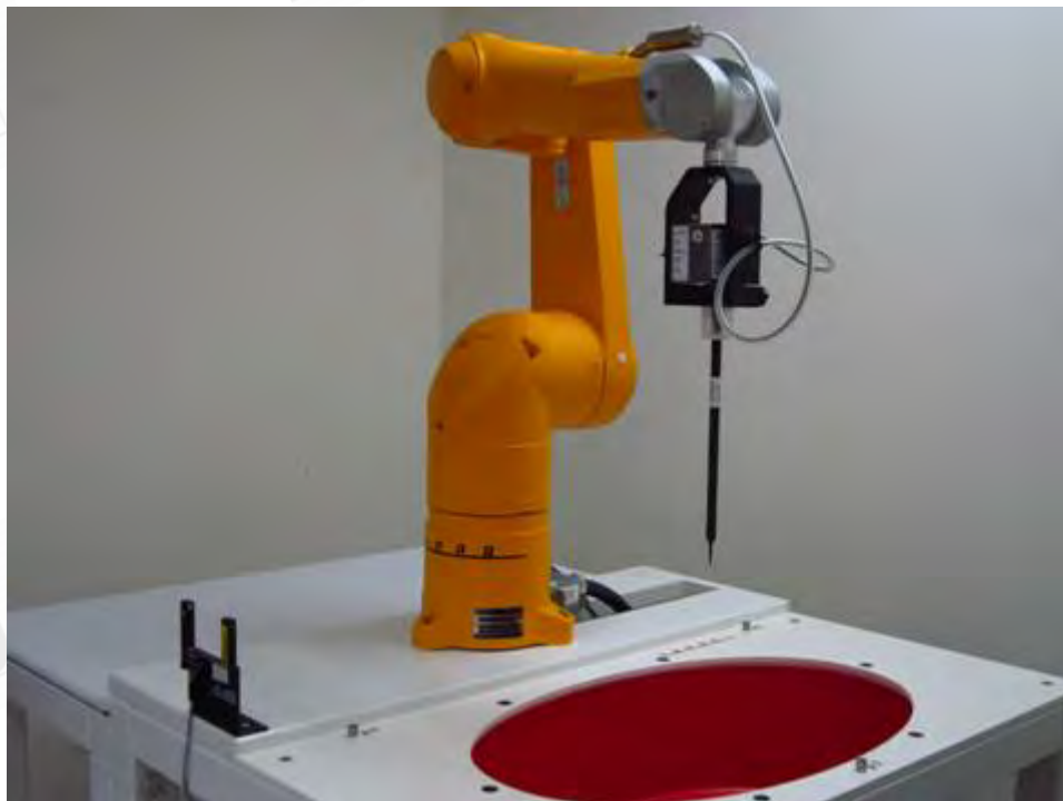
Fig.1 Photograph of the SAR measurement system
