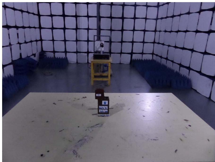
**Radiation Emission Test Setup (30MHz to 1GHz)***Test Mode: Only Charging*
