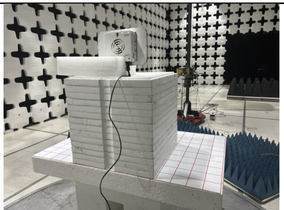
Radiated Emission Test 1-18GHz Rear View
