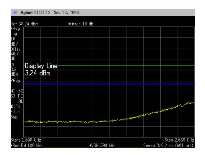
\* Blue limit line is from 74.637 (a)(iii): 43+10log<sub>10</sub>(P<sub>Mean</sub> in watts)
