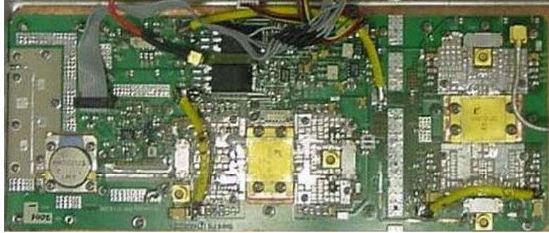
1.99-2.5GHz Power Amplifier Board (PA) 7214208000
