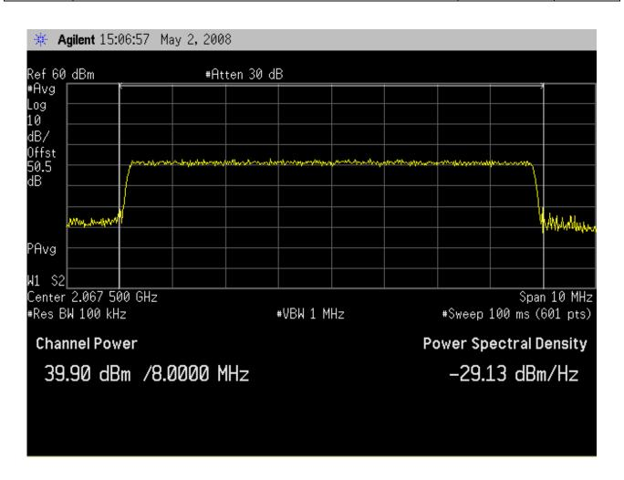
Average Measurement (64QAM 8MHz 2067,5MHz) 39.90 dBm = 9.77 Watts
