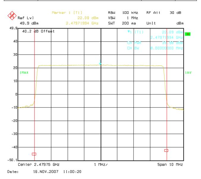
Average Measurement (64QAM High Channel 2450 to 2483.5 MHz Band)
