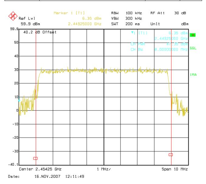
Peak Measurement (QPSK Low Channel 2450 to 2483.5 MHz Band)
