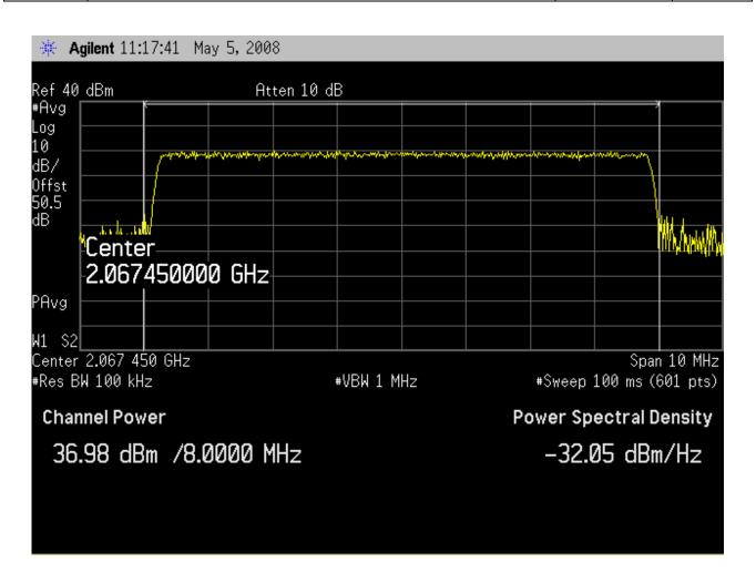
Average Measurement (64QAM 8MHz 2067,5MHz) 36.98 dBm = 4.98 Watts
