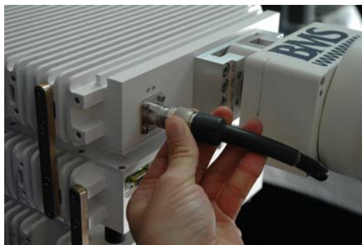
Figure 12 Connect the RF Cable to the RF In Connector on the FCII-MAX
