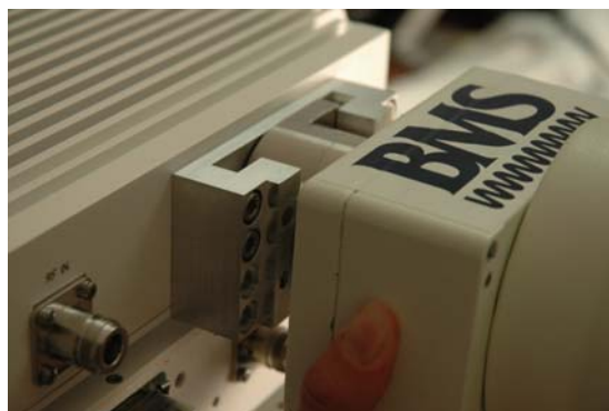
Figure 10 Antenna Locked to Mount
