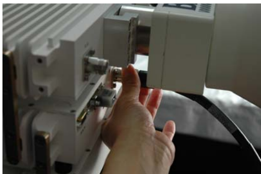
Figure 11 Connect the RF Cable to the FCII
