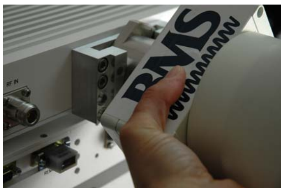
Figure 9 Rotate Antenna to Lock
