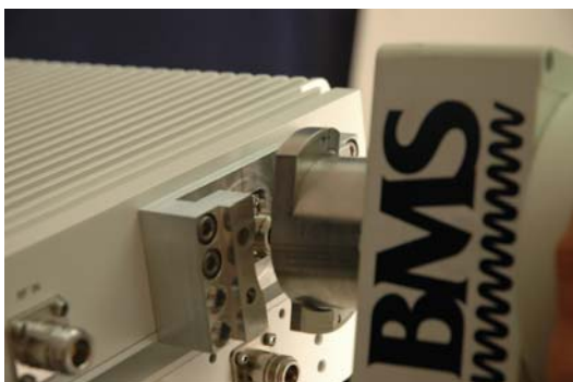
Figure 7 Align Antenna Mount with Bracket
