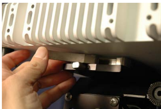
Figure 4 Figure 4 Fold the lever flush
