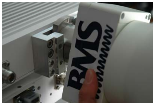
Figure 8 Insert Antenna Mount into Bracket
