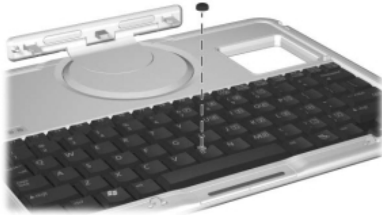
Replacing the pointing stick cap
