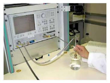
Tissue used during the SAR assessment is calibrated prior to in the measurement use process. APREL Laboratories use the co-axial probe method for all tissue calibration exercises. Tissue which is being used over a period of 24 hours is recalibrated to ensure that no change to the dielectric properties will affect the SAR measurement process. The table below provides details of the tissue results from the equivalent dielectric calibration.
