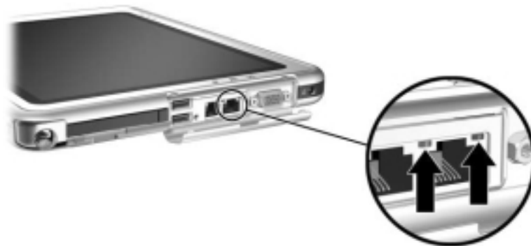
Identifying the LAN connection lights
