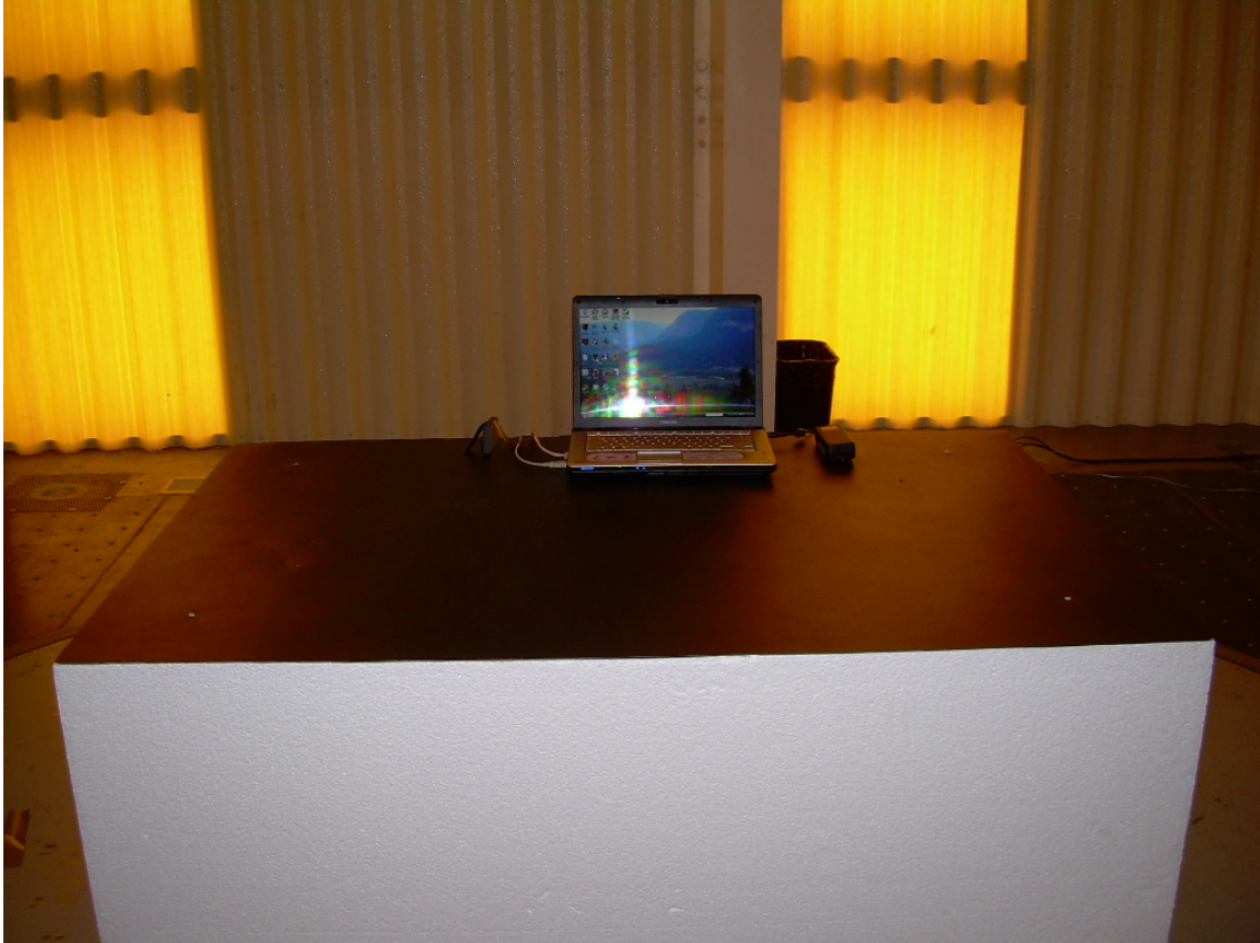
Photograph 2 - Front View Radiated Test Setup - On-Edge EUT Placement
