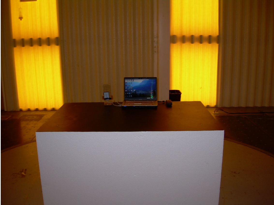
Photograph 3 - Front View Radiated Test Setup - Vertical EUT Placement
