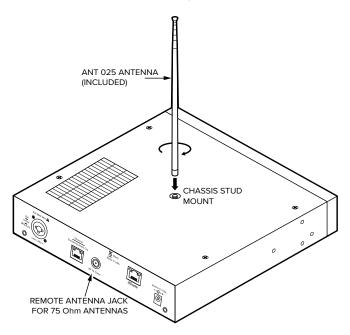
NOTE: If the FM + C is going to be rack mounted, you will not be able to install the ANT 025 whip antenna. For rack mounting, consider installing a remote antenna like the ANT 005 or ANT 024 - these antennas require using the Remote Antenna Coaxial Jack (above) and a long length of terminated coaxial cable. Another option is to mount the antenna on the rack itself - consider the ANT 029 which includes a 1RU bracket and a 3ft terminated coaxial cable.
