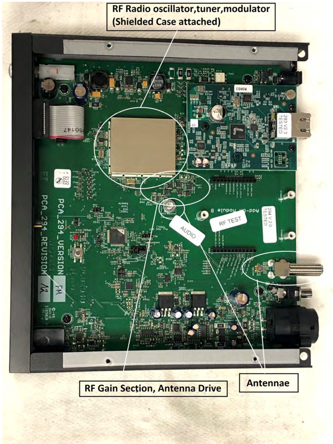
Photo1: Internal Top view of system main board (PCA 294) installed in chassis, and showing location of key RF radio sections.
