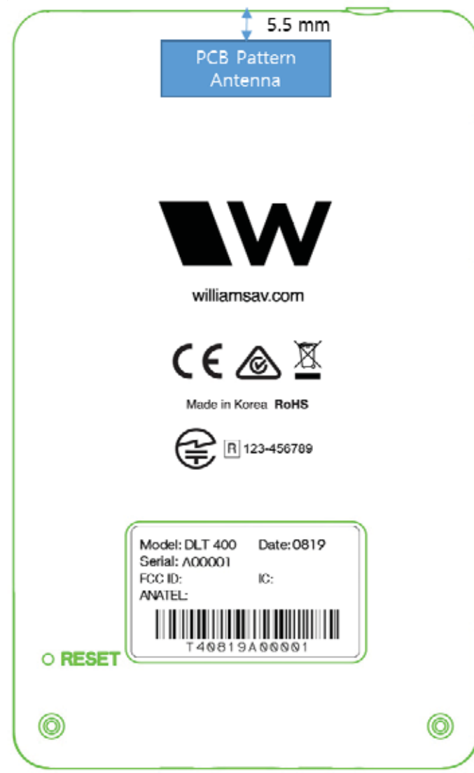
Figure F-1 Antenna Location
