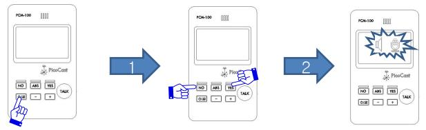
Press and hold power button for 2 seconds to turn DLT-100 on Press No and Yes button together for 2 second
