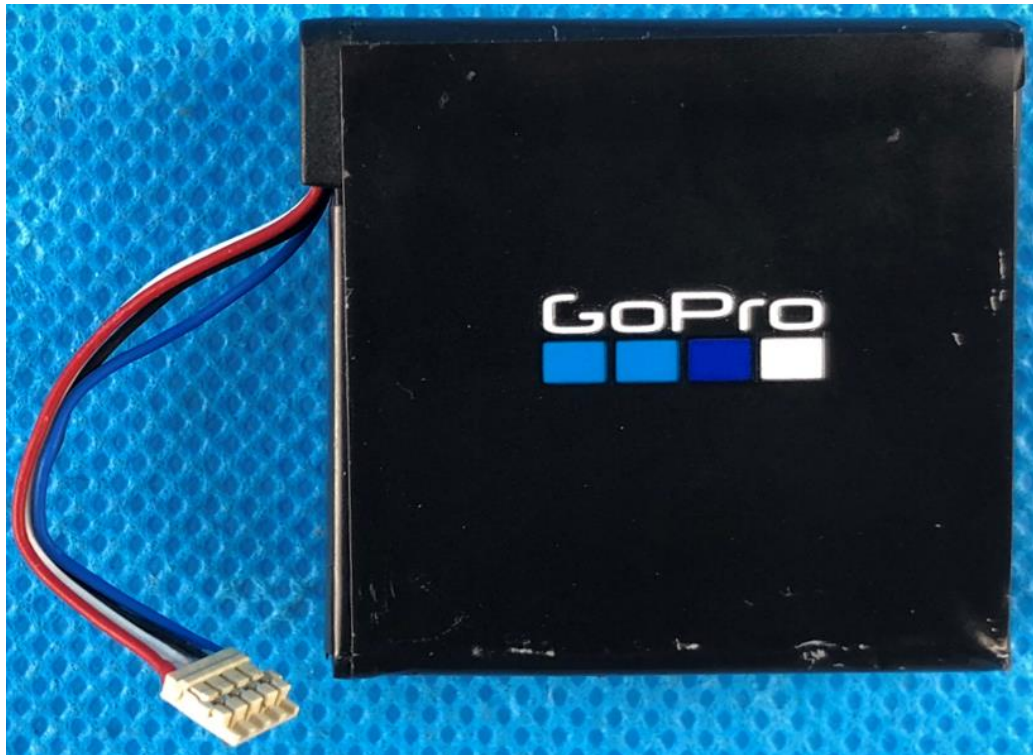
SPTM1B, lithium battery- SPTM1(Version S and Version W) -Front
