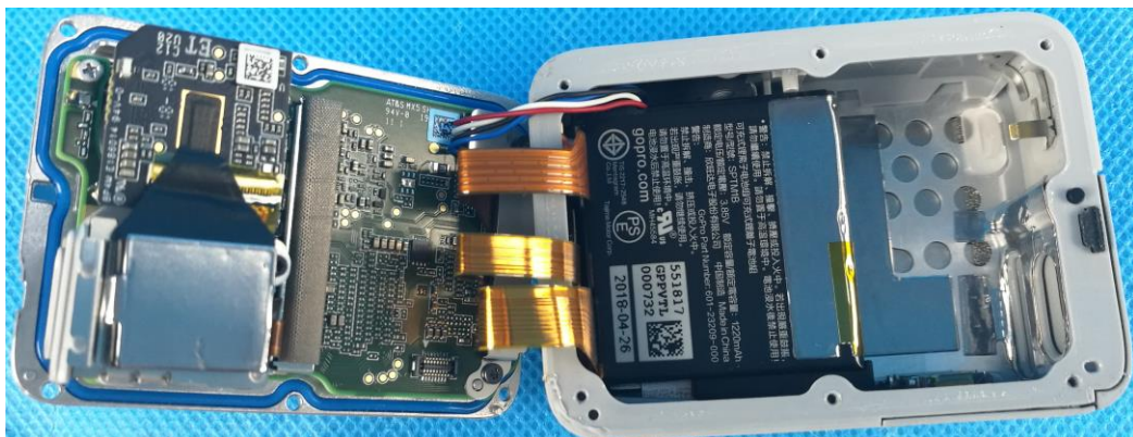
SPTM1 (Version W) heat sink removed
