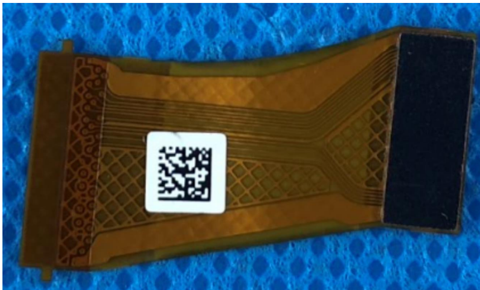
656-22984-000 FPC, JUMPER, IMAGE SENSOR- SPTM1(Version S and Version W) -Back
